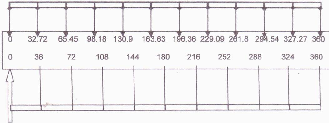
Ten coils at 36 degrees interval shows the gaps in degrees
