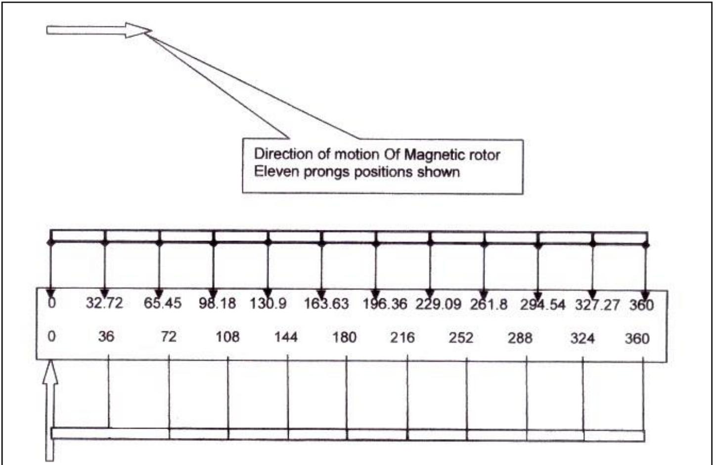
Ten coils at 36-degree intervals show the gaps in degrees when both prong and coil are aligned at  $0^\circ$ . It is the position at which a polarity-reversing impulse is given and it shows that none of the other ten prongs are in line with any of the nine other coil core centres.
