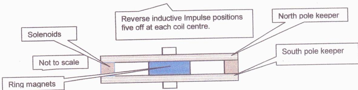
Plan view shows ring magnet at centre and opposed wound solenoids at boundary. The keeper plates with prongs and ring magnets rotate past fixed solenoids. Timed impulse maintains rotation. Solenoid coils generate current.
