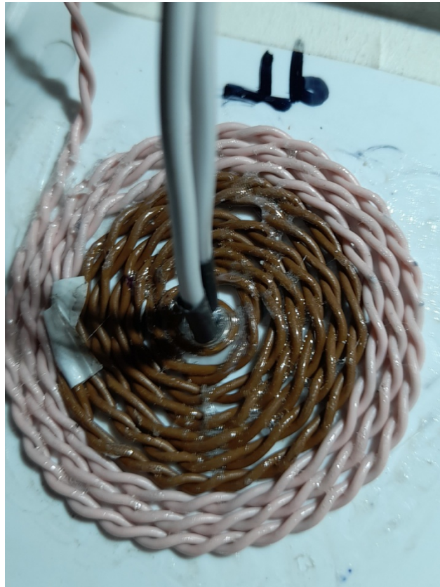
Mobius coil example, 9 turns with LED at centre
