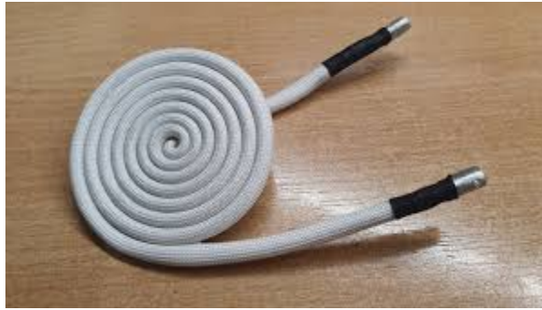
Pancake coil for pots, outer connection goes to 1 st pot
