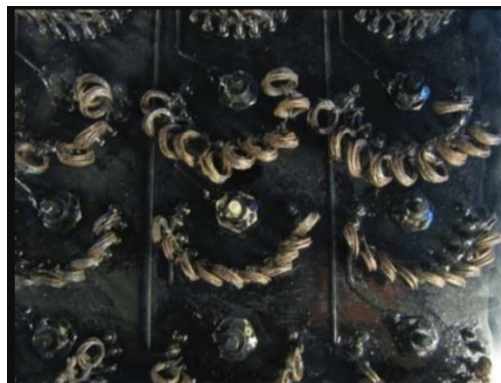
Original Abrams resistor box with 1 ohm coils as resistors
