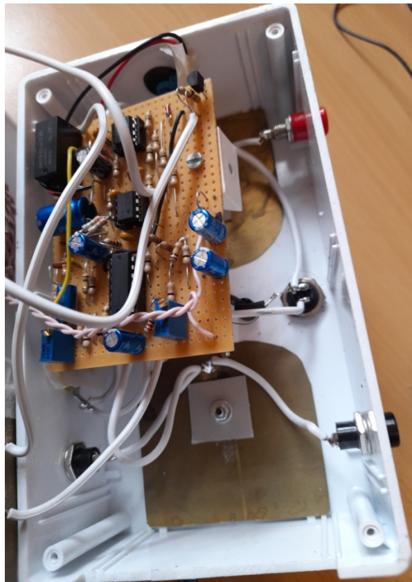
Brass input and output plates with Vero board for the circuit
